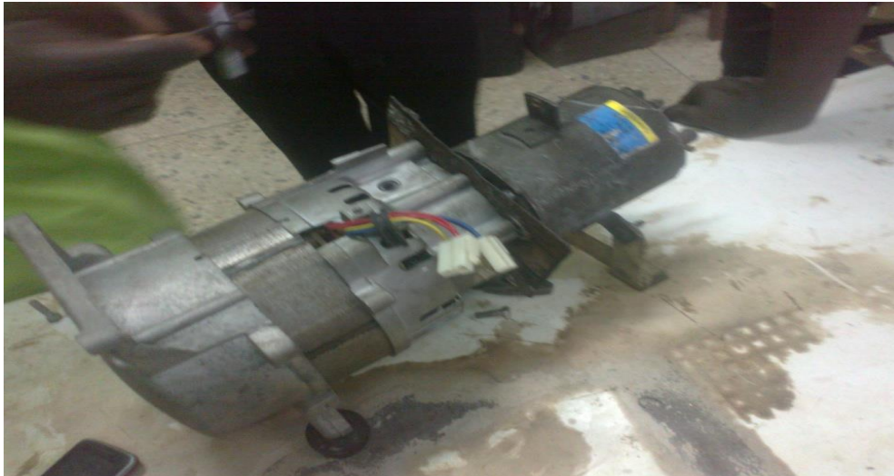
Figure 8 Mounting of the DC motor to alternator
